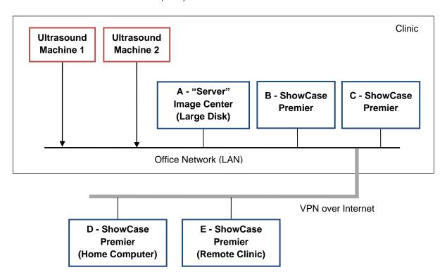
The Ultrasound Machines send study data to the **A** "Server" computer running ShowCase Image Center. The Image Center stores the study data to a large disk. ShowCase Premier on computers **B** and **C** is configured to access the Image Center directly, as local viewers. ShowCase Premier on computers **D** and **E** are configured to access the Image Center over a VPN, as remote viewers. The Image Center can store up to 200,000+ studies.
